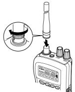
To attach the supplied flexible antenna to the connector on the top of your scanner, align the slots around the antenna's connector with the tabs on the scanner's BNC connector. Then slide the antenna's
